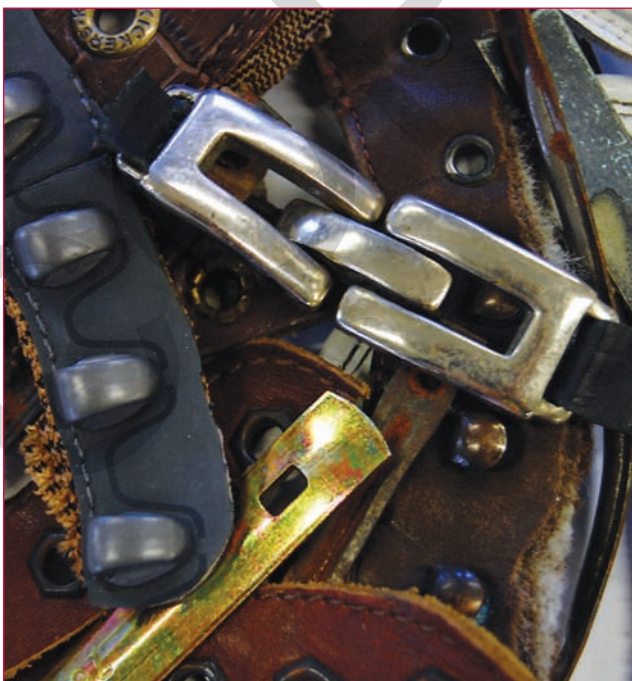
Typical metallic items found in footwear. Steel shanks moulded into soles are particularly difficult to extract.
