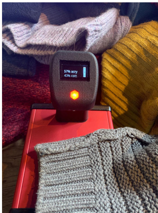
Image 9: Composition scan using Matoha NIR handheld scanner (Source: Matoha)
