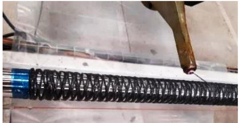
Figure 5: Filament winding with the recycled yarn
