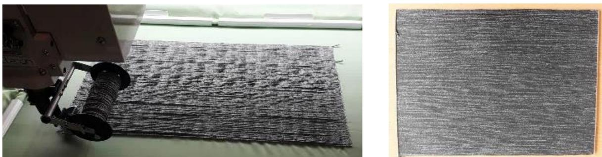
*Figure 3: Manufacturing of the yarn/epoxy composite plate for mechanical characterisation*
