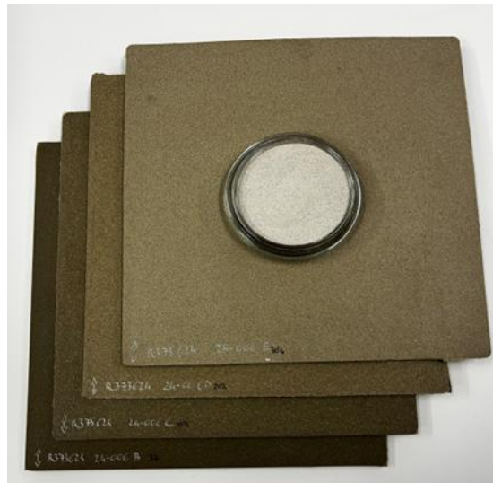
Figure 33: Micronized rubber (on top) and plates containing different rates of micronized rubber
