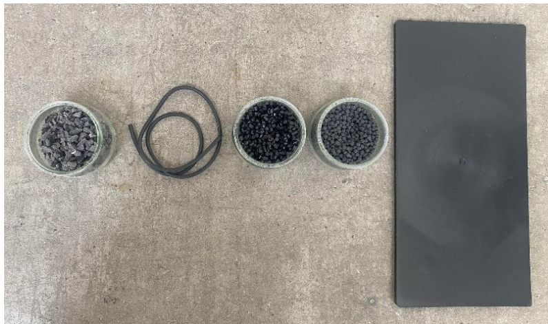
Figure 29 : From left to right: ground material, extrusion rod, recycled pellets, virgin pellets and injected plate containing 50% recycled material
