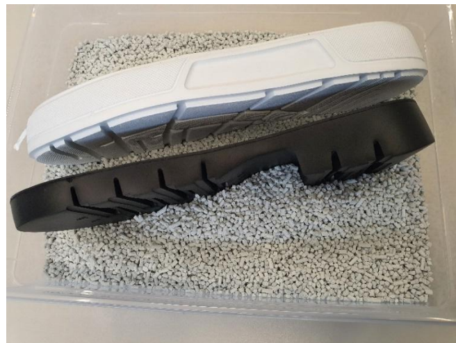
Figure 18 : Soles produced in using recycled EVA by Viriam
