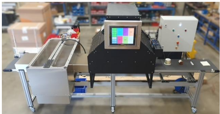
Figure 5: Sorting line using a hyperspectral camera - Plas'tri 16
