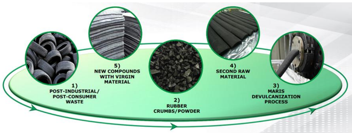
Figure 22: Maris recycling process integration diagram (source mariscorp.com)
